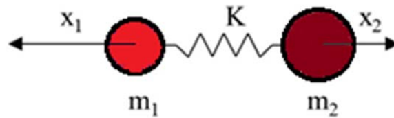
Fig. 2: Diatomic molecule as a mass on a spring.
